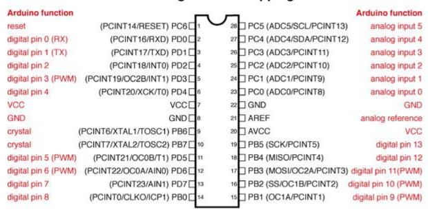
Digital Pins 11,12 & 13 are used by the ICSP header for MOSI, MISO, SCK connections (Atmega168 pins 17,18 & 19). Avoid low-impedance loads on these pins when using the ICSP header.
