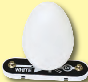
Egg LED attachment mounted to D6
