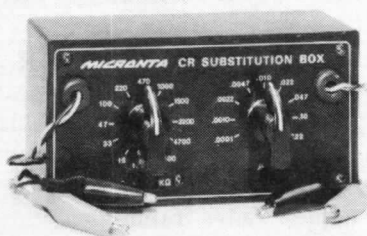
Figure 5-14. A resistance-capacitance substitution box.
