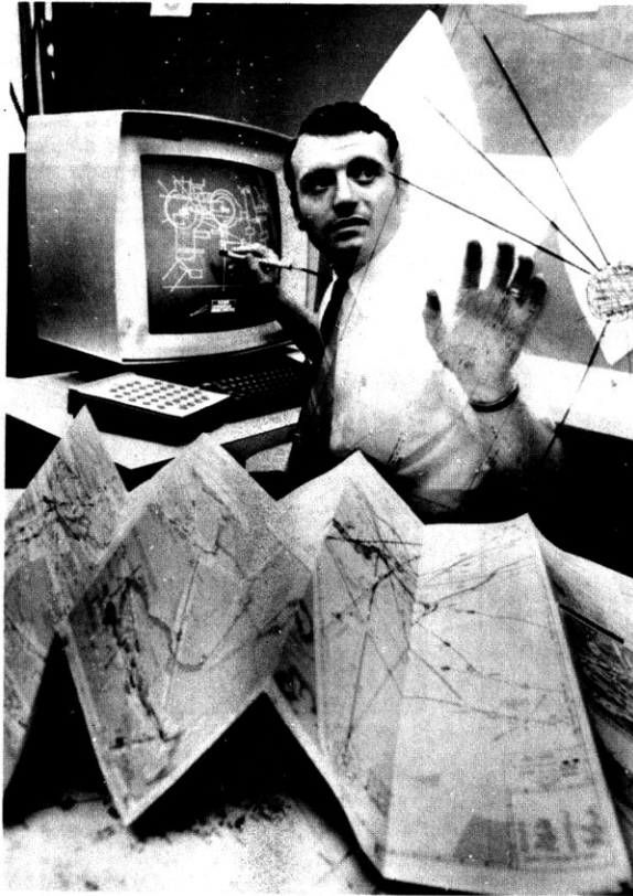
This person is using a light pen and a typewriter-type device for input. Output appears on the screen.
