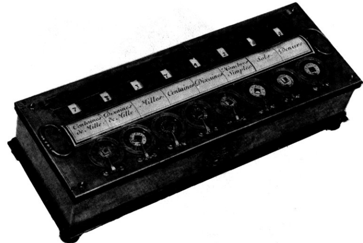
Pascal's calculator invented about 1640. Its gears carry the "tens" over to the next column.
